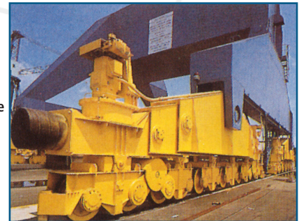
Cellular buffers at the travel unit of a 200 t shipyard crane
