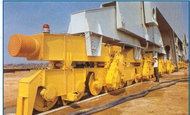
Cellular buffers at the travel unit of a 900 t gantry crane
